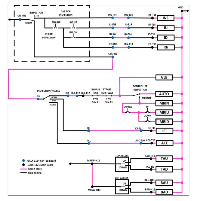
Figure 3-3: Inspection String Circuit
