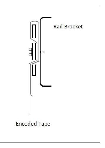
Figure 2-2: Front View of Encoded Tape
