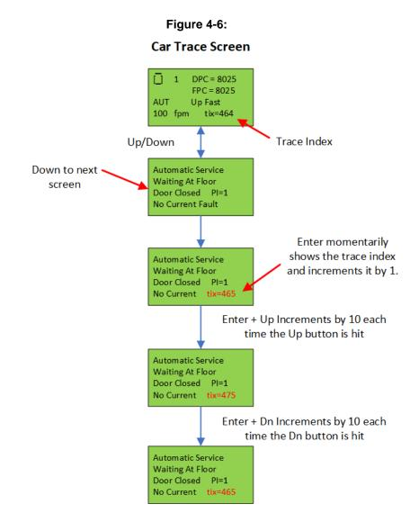
To navigate the trace screens, hit the UP or DOWN buttons to change to the next status screen. To increment to the next trace frame, hit the ENTER button. Hitting the ENTER button will cause the trace index to increment by 1. To increment or decrement quickly through each frame, hit and hold the ENTER button and then hit the UP button to increment the index by 10 or the DOWN button to decrement by 10.
