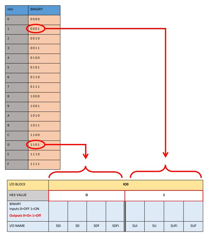
Place the Binary value for D (1101) in the first four bit locations and then place the binary value for 1 (0001) in the last four bit locations.
