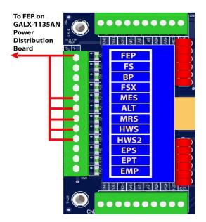
Figure 3-0: Typical I/O Expansion Board Fire I/O Board
