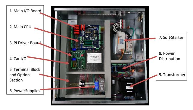
Figure 1-0: Typical Physical Layout of Top Cabinet
