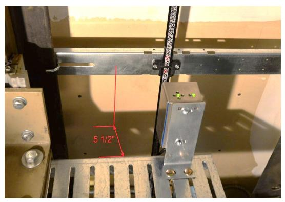
Figure 2-10: APS Camera and Mounting Bracket
