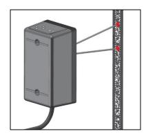
Figure 2-15: APS Camera Alignment Spotlights
