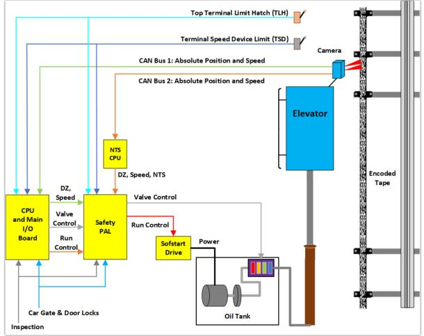
Figure 1-1: Absolute Position System Selector
