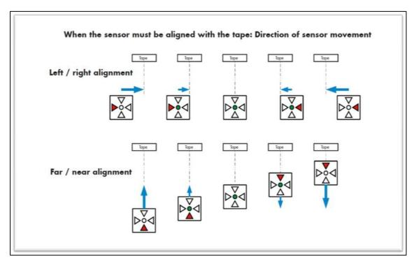
Figure 2-16: Fine Adjustment of the Camera Sensor
