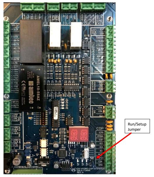
Figure 2-19: GALX-1134AN COP Interface Board Setup Jumper
