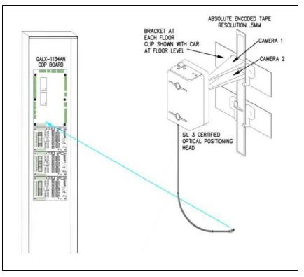
Figure 2-13: Wire APS Camera According to Wiring Schematic and Connection Diagram
