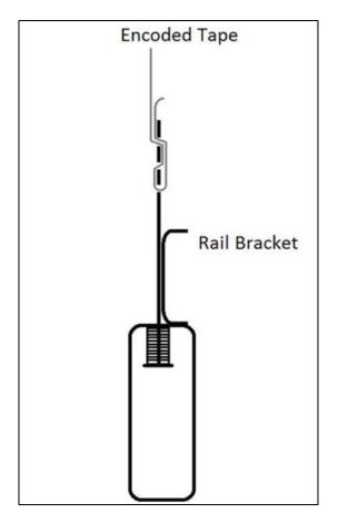
Figure 2-8: Side View of Encoded Tape Attachment to the Bottom Bracket
