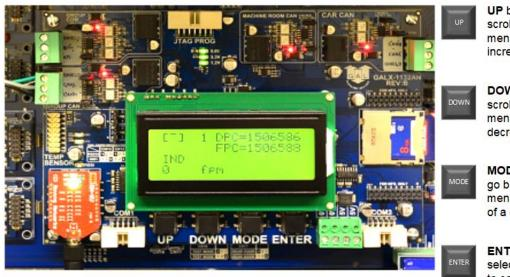
**UP** button is used to scroll up to the next menu item or to increment a data value.
