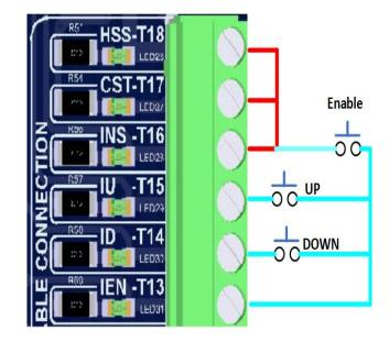
Figure 3-1: GALX-1121 Main I/O Board With Run Bug. See Figure 3-2 For Run Bug Stop Switch.
