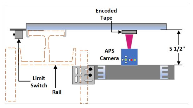
Figure 2-11: Top View of APS Camera and Mounting Bracket
