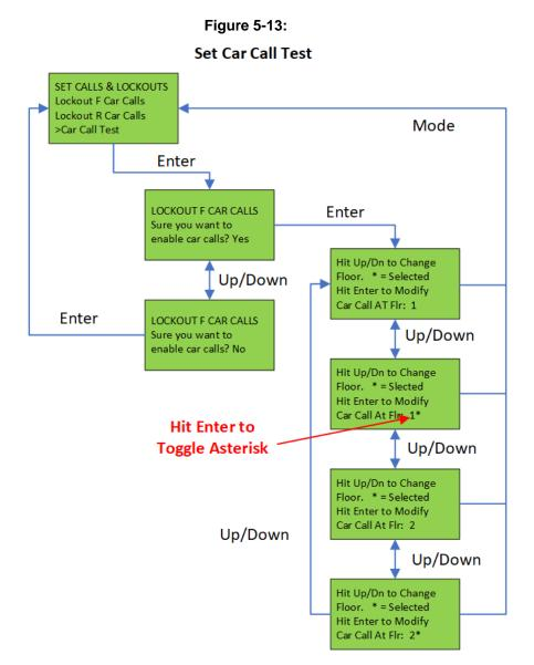
This operation will continue until the test is discontinued from the LCD interface, the car is taken out of automatic operation, or a fault occurs.
